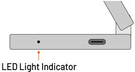
FOD (Foreign Object Detection)/Malfunction: Blinking blue land red light.—) —
